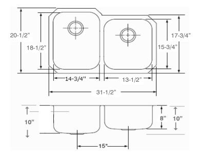
Installer Notes: Ukinox always recommends that you give the sink to the granite fabricator. If you are going to use a cutting board, provide that to the fabricator as well. Please note that we do include a template with each sink, but there can always be a slight variation. In addition, many of our templates are perforated so you can tear off the perforation for cutting board applications.
